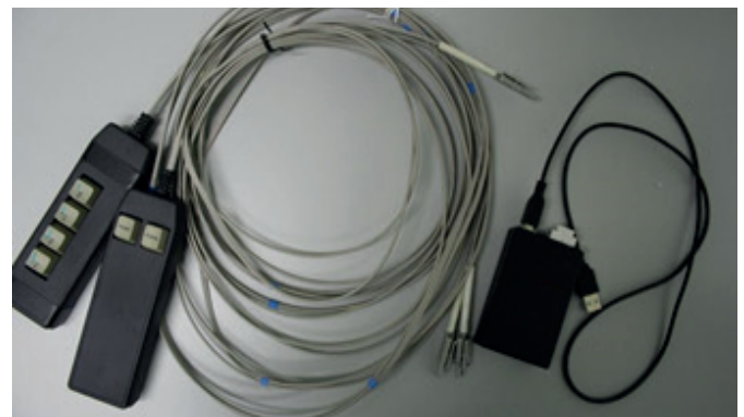
A set for recording reactions during measurement in a rTMS laboratory
