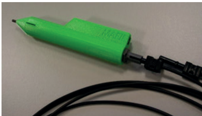
MR compatible pencil - designed for recording measured person's responses
