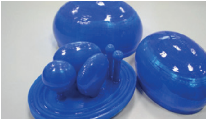
Shepp-Logan phantom - a multicompart ment phantom that is used as a model of human head
